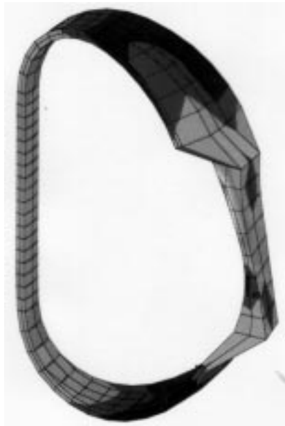
Figure 6.5-15. Stresses in the external coil structure for the third model, with 1.2 GPa maximum stress in the region where the cap stops.
