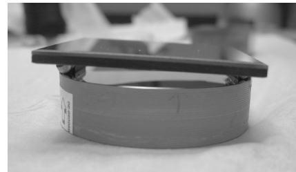
Figure 4. Simulated monolithic wedged dichroic mirror (2-in diameter)
