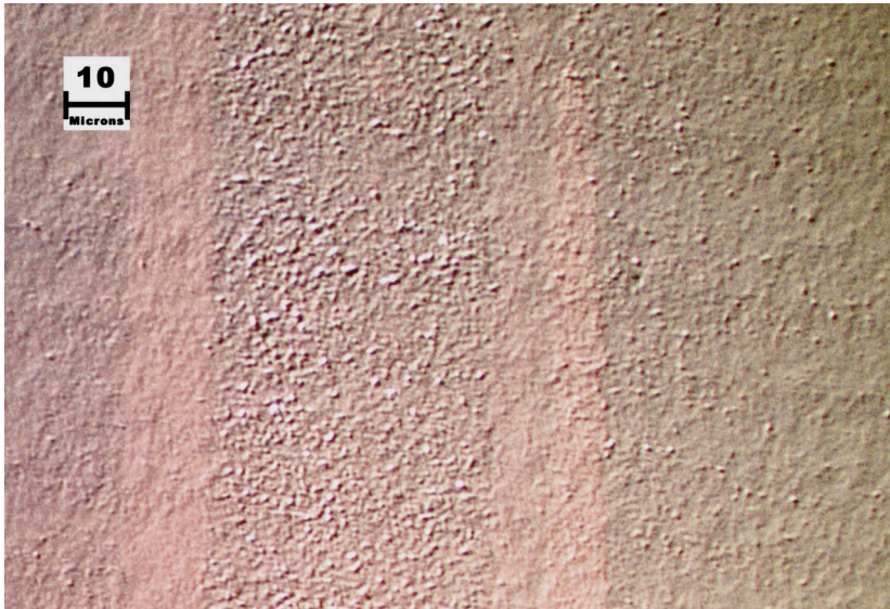
Fig. 10. Typical high-cycle damage (400X)
