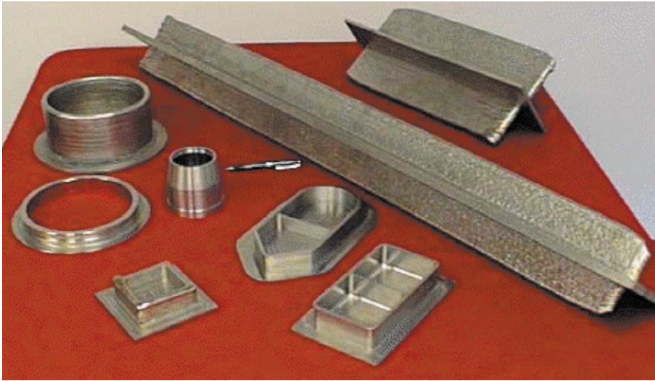
Fig. 5. Typical laser-formed parts produced by AeroMet.
