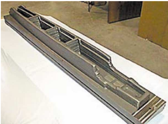
Fig. 6. An as-formed titanium part illustrating the laser forming condition.
