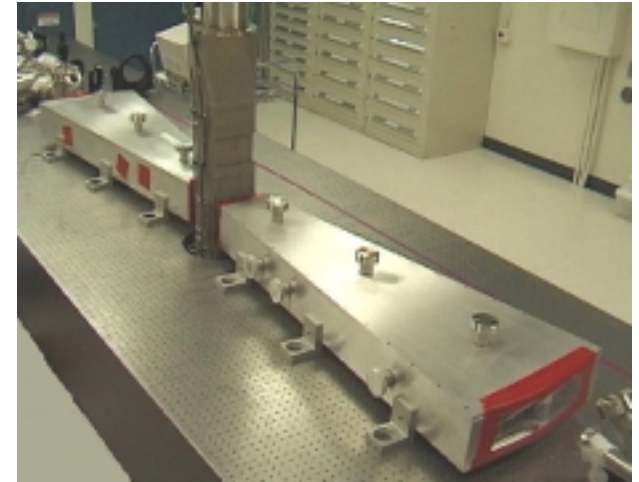
Gas-cooled amplifier heads • He gas flow at 0.1 Mach
