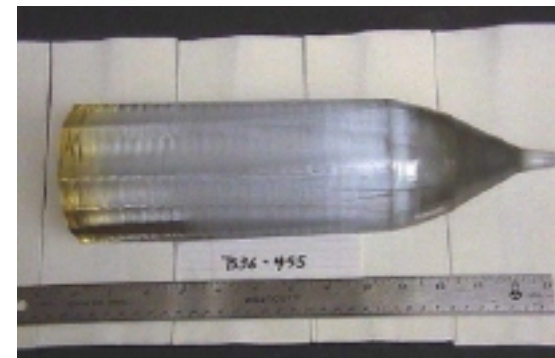
5 inch diameter Nd:GGG crystal grown by the flat interface method.
