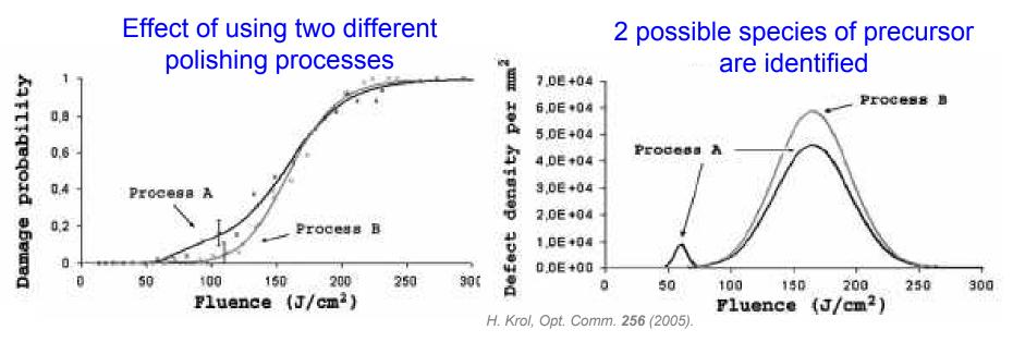
Phenomenological models can be used to help interpret the damage test data and help identify possible causes of damage initiation
