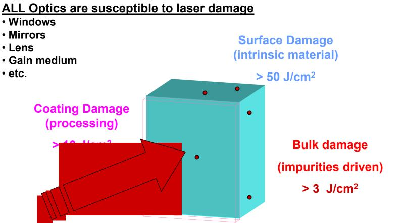
All optics (regardless of laser type) subjected to laser illumination will suffer from wear and tear and are susceptible to damage eventually.
