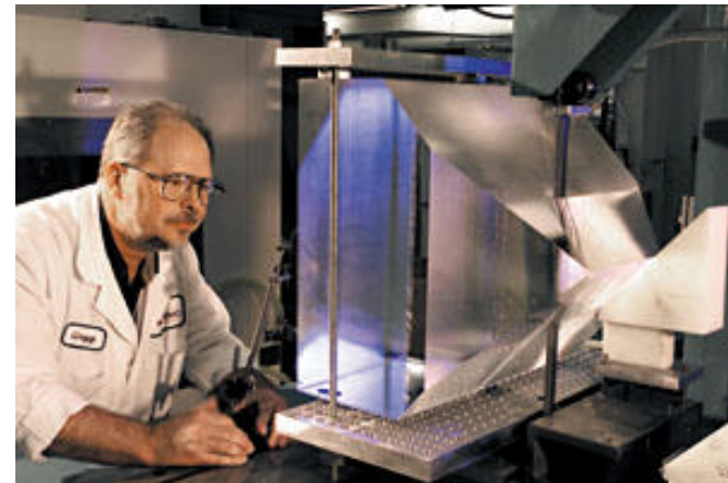
DKDP is harder to grow than KDP but 80% DKDP has been grown to 40 cm apertures
