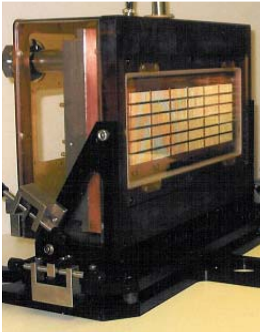
Diode pump arrays
