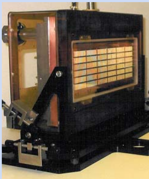
80 kW pump diode arrays
