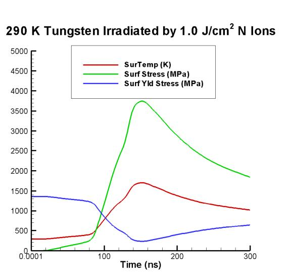
At peak surface temperature, 2.5 µm of material is yielding 290 K Tungsten Irradiated by 1.0 J/cm<sup>2</sup> N lons
