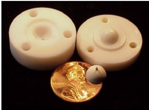
4 mm diameter hemishell - 400 \mu m wall
